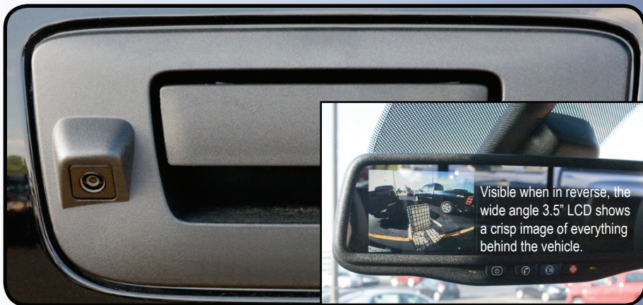
Gate-mounted backup camera with integrated 3.5" LCD Rearview Mirror. A popular option for buyers of new Chevy Silverados and GMC Sierras.
